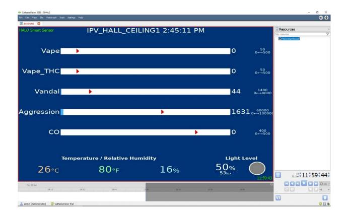
Drag the HALO Smart Sensor device from the Right navigation tree into the Viewing panel of the CathexisVision Client to visualize the live, real-time output from the HALO Smart Sensor.
